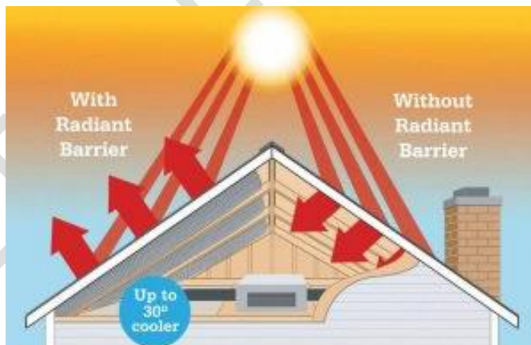
Plate 15: Thermally cool roof interiors analysis (For reference purpose only)
